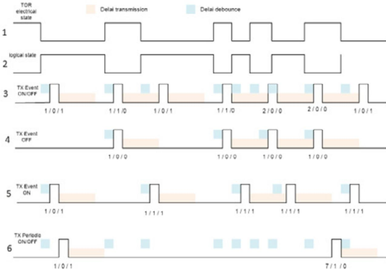
The 3 figures under the pulses are: the number of events / the previous state / the current state.
