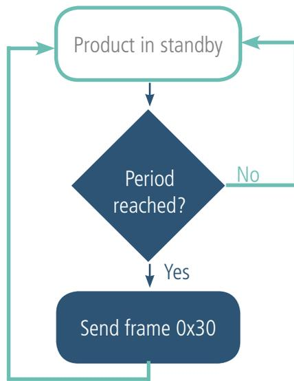
If one of the inputs is in periodic mode there is no Keep Alive frame transmission.
