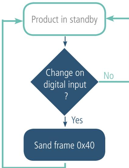
The monitoring of events on the enabled inputs continues even during transmission of the frame.
