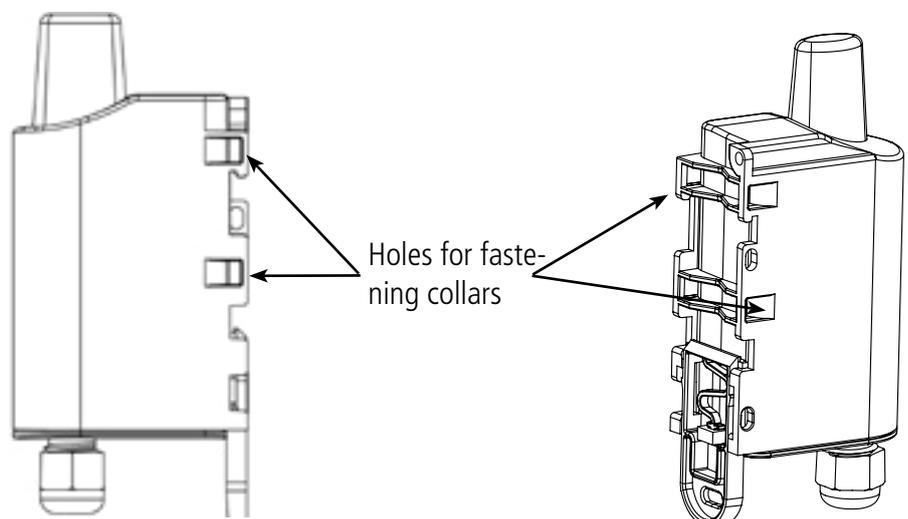
To optimise fastening onto a tube or mast, we recommend you remove the Rail-DIN locking/unlocking lever.
