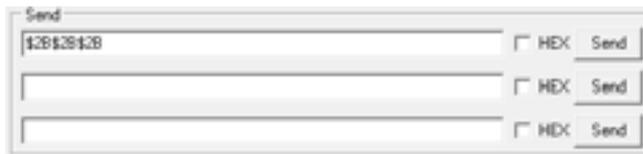
Send the transition frame in command mode in order to switch the device to configuration mode by clicking on the SEND button.
